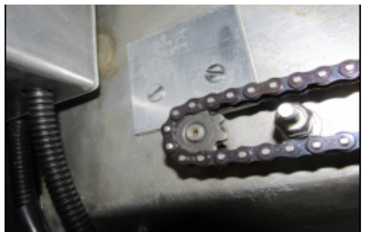
Driven sprocket on fuel tap shaft
