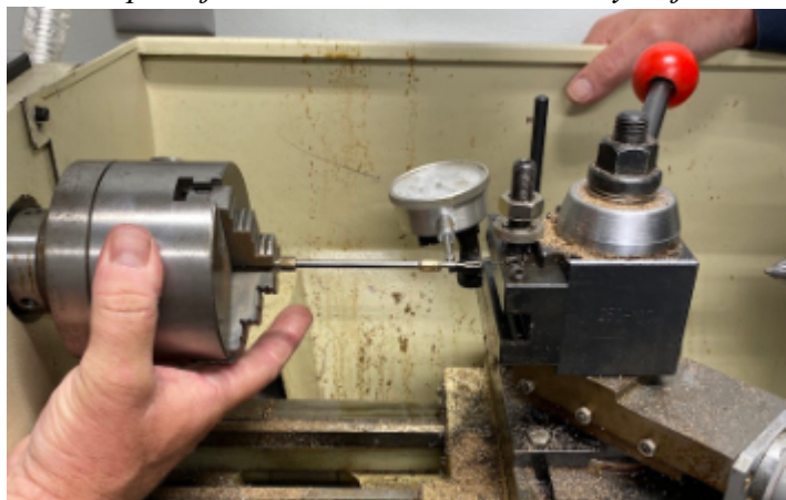
Needle chucked in lathe shows it is bent
