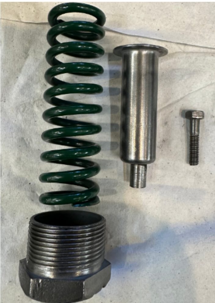
Left: New "Heavy" springs and the guides dismantled. The stamped guide has been trued and new top hats have been turned. "Past Practice" says never take the spring packs apart. Based on new knowledge, they should be checked. But will require a spring tester to reassemble!
