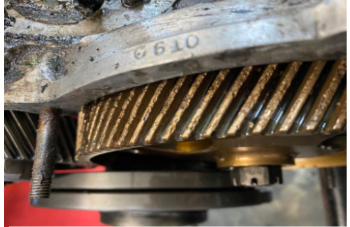
Bronze timing gear with pitting due to tight meshing
