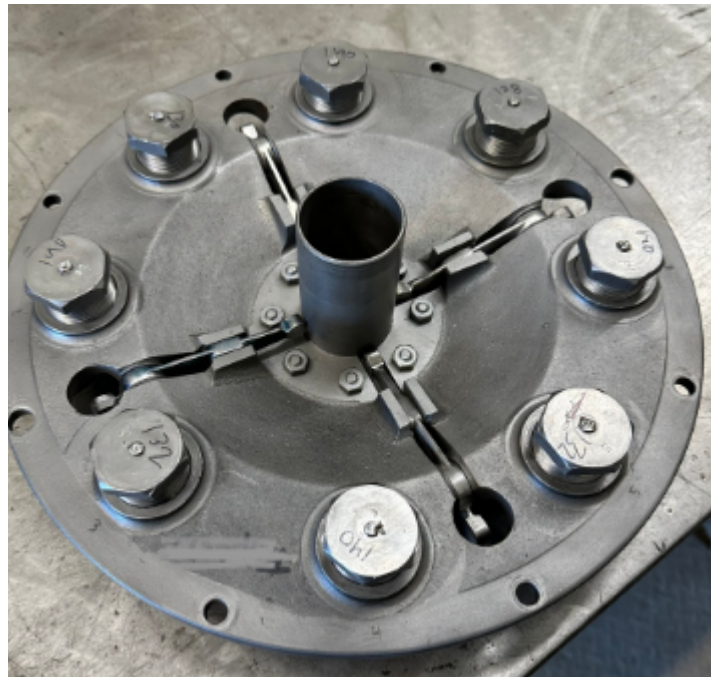
Tested springs in place. Note that large HP cars have shim washers included with them. Small HP do not. Springs are within about 5 percent of each other. All tested before peening the ends.
