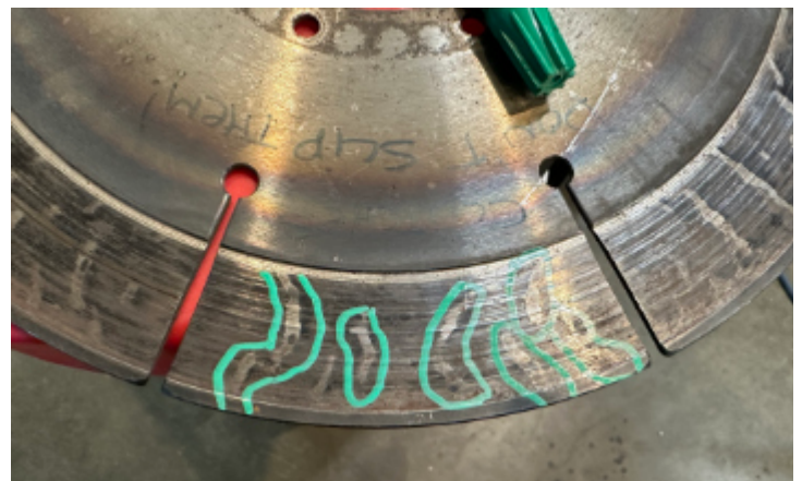
Severely overheated clutch plate showing hard areas (circled in green) These are raised above the softer (worn away) area. These high spots lower the contact area of the clutch and create slipping and, by extension, more heat and wear.
