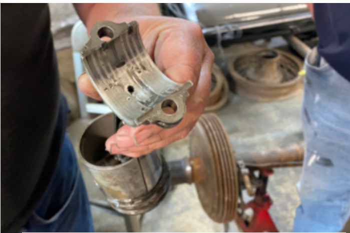
Dual thin shell bearings in rod, instead of babbitt
