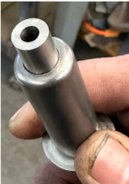
Note nice fit of the new top hat to the guide
