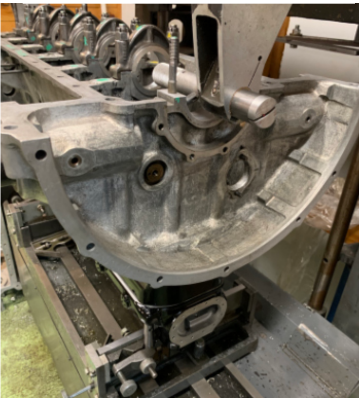
Line boring new main bearings
