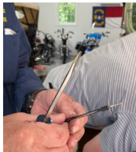
Bent low speed jet needle
