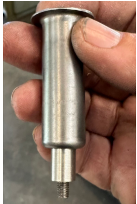
New guide with new top hat fitted together. Just a few thousandths of clearance, not large wear/slop.
