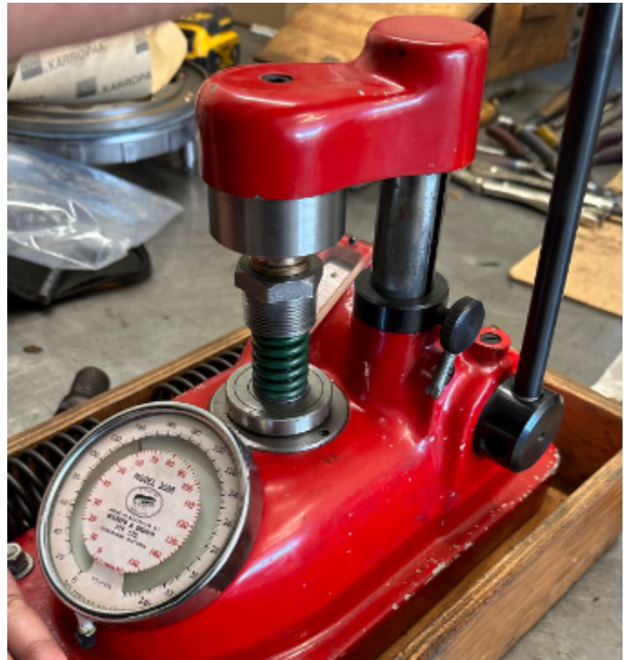
Using a spring tester to make sure all the spring packs are going to put equal pressure on the clutch
