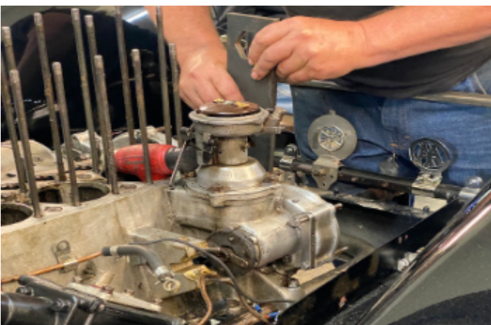
Slogging bar to remove crankshaft pulley nut
