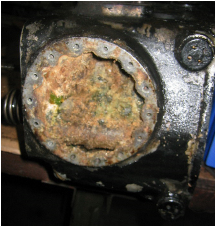
Head full of Bar's Leaks. This is an extreme example of an owner trying to avoid addressing the head by continuing to pour Bar's Leaks into the head until the entire water chamber was plugged. The car actually ran quite well!
