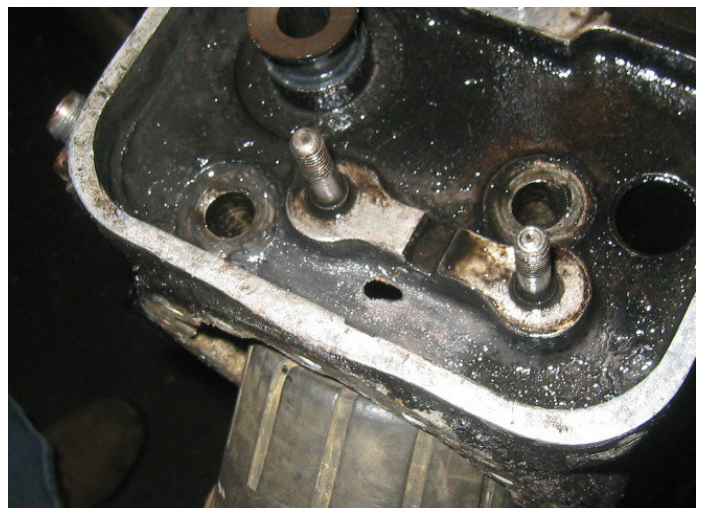
Head rusted through from inside. Here is a Large HP aluminum head, rotted through from the inside. From the outside, head looks great. They dissolve from the inside out! Same is true of iron heads.
