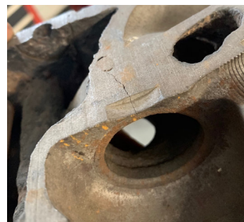
Crack in the combustion chamber. Probably caused by freezing. External freeze cracks can often be repaired with pinning. But internal cracks are a non-starter.
