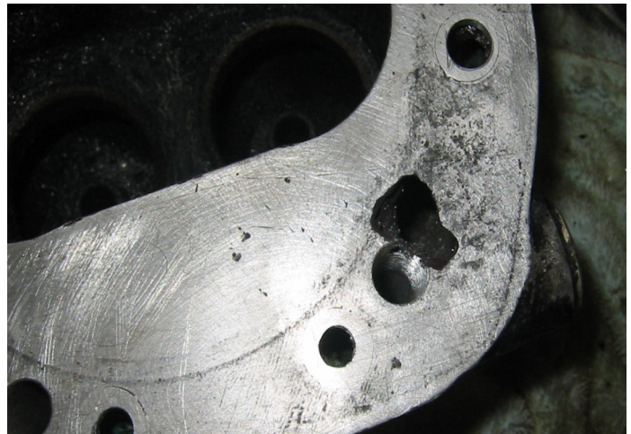
Another picture of a head rotted through from the inside. Are we seeing a theme here?
