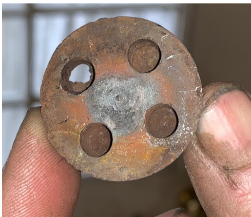
This is a core plug that has rusted through from the inside. While it looks solid, the rust from behind has eaten its way all the way into the hole for the pin spanner. If this is going on, inspect all plugs and replace them all. They are not cheap, but losing all your water externally or, worse, internally, costs a lot more!
