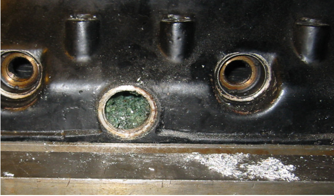
Another head full of Bar's Leaks and aluminum oxide that has rotted off the casting. Once a head is rotted this badly, there is no repairing it.
