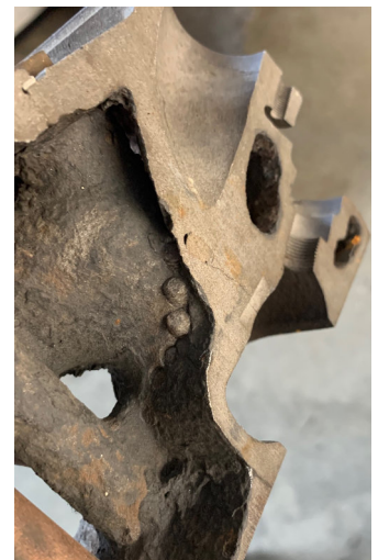
This head has a serious crack in the combustion chamber and an attempt has been made to pin it using hardware store bolts and screws. Needless to say, it failed immediately. Head has been sectioned to show the 'bodge' repairs and the extent of the crack, which extended behind the valve seat.
