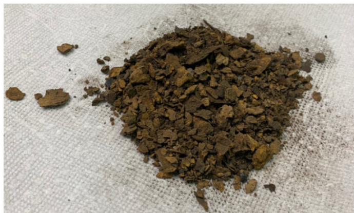
This is just a fraction of the scale, rust, lime and other detritus that came out of a small HP block. Essentially the 'loose' material, the entire contents filled a coffee can.
