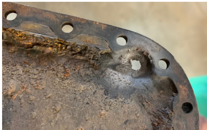
This is a small HP water jacket cover after bead blasting away the rust/scale. A large hole was lurking just under the surface. Water being held in by paint and a thin ‘foil’ of metal. Paint is not intended to be structural.
