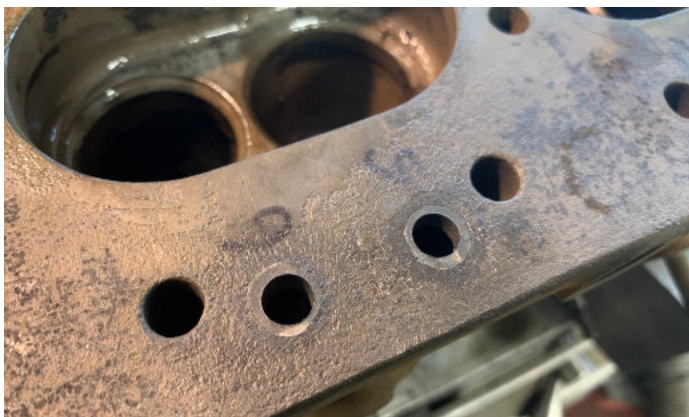
Repaired water passage. In this case, in a cylinder head. But a block repair is simply the mirror of this and must be done before putting that nice new head on. Otherwise, your head gasket will not seal. Period.
