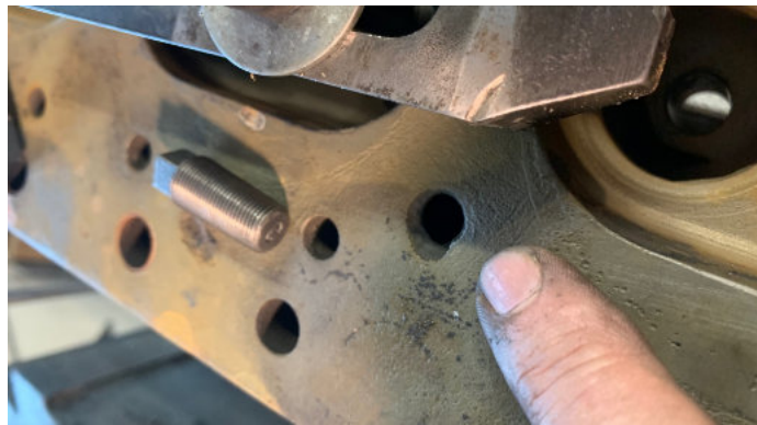
Note the severe erosion around this water passage. These must be clean and sharp. While this is a cylinder head, the same applies to a block when it comes to an eroded water passage. The edges of the passages need to be sharp and consist of good cast iron, not crumbly rust. We repair this with a tapered plug which is then decked smooth and re-drilled to create a good head gasket seal.
