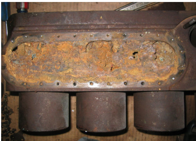
This is a badly scaled-up small HP block. Several pounds of lime, scale and rust displaced water, insulated cylinder walls and stopped circulation. Do NOT under any circumstances put a new cylinder head on a block that looks... like this!
