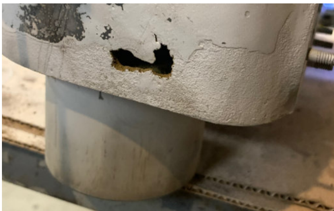
This block looked great until the scale and lime was cleaned out of it. But the lime and scale were hiding a thin spot that revealed itself while bead blasting. Probably an old flaw in the original casting – a bubble. But it managed to last for some 80 years before failing. New block, unfortunately, was required.
