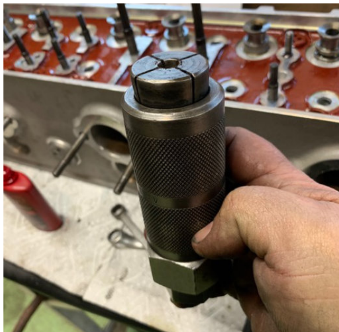
This is a collet-style stud puller/fitter. Hard to find and expensive on places like eBay, it is worth its weight in gold when fitting studs in a new head. Or removing them...
