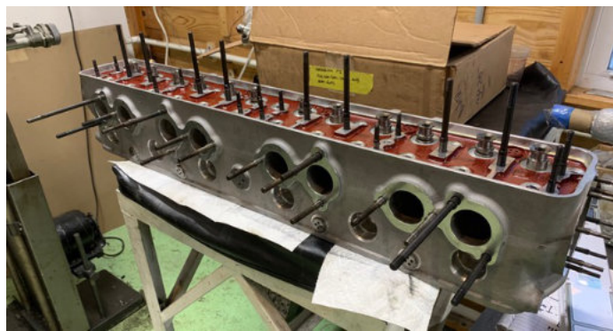
Head with all studs ready to fit. Note that they are threaded in only as far as they will go with 'finger pressure.' In other words... they need some fitting by chasing both male and female threads. Studs should screw in basically with finger pressure before final tightening.
