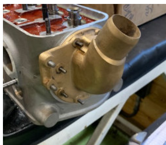
Front cover temporarily fitted. Make sure gasket faces are clean and at gasket with sealant. We use a non-silicone sealant here because the head is unpainted. If we used a silicone sealant, the paint would be a mess!
