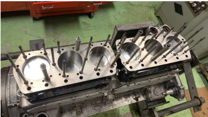
Block surfaces before fitting. Note that water passages have been bushed and that the blocks are being held in place with spacers to protect the base gaskets.
