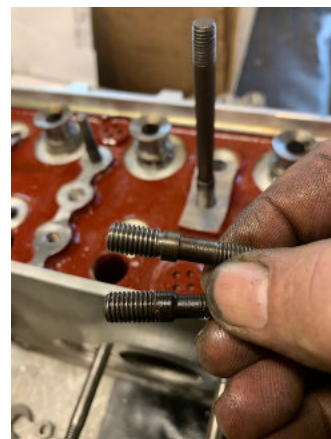
Stud on the bottom is 'as taken from the parts bin.' On the top is after chasing, wire brushing and some lathe work to clean up a gap under the step. This ensures the stud seats fully and cleanly at exactly the right depth. It's more than just screwing things in!
