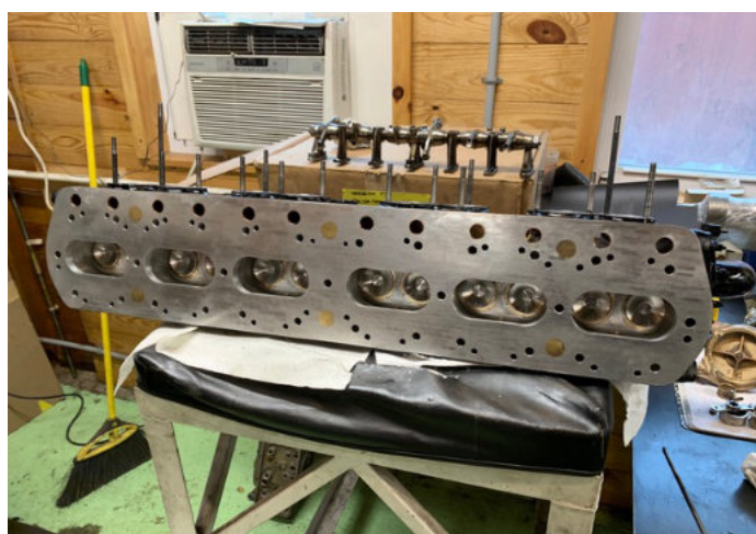
Head ready to go on. De-burred, painted, with valves in place and all studs fitted. Note how the face has been protected and is free of scratches, nicks or burrs.
