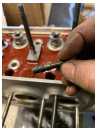
Stud ready to fit. Chased, machined and burnished so it is smooth.
