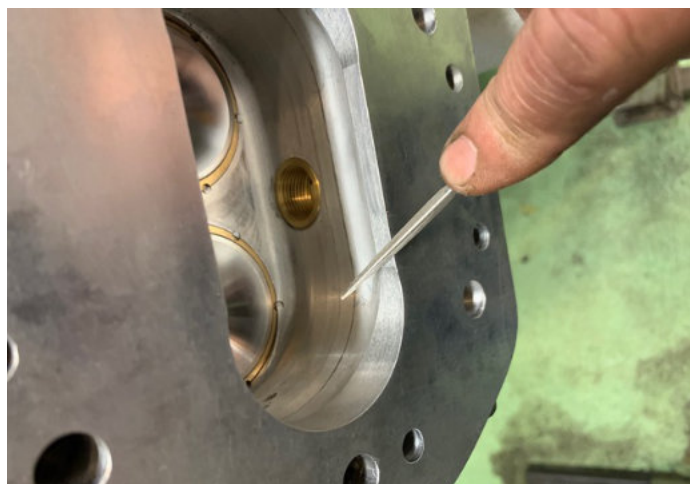
Just before fitting, we ran our fingers over the casting and found a few wire-edges on the edges of the combustion chamber. Your fingers are more sensitive than your eyes when it comes to finding burrs and anomalies. A fine Swiss File cleaned up the burrs.
