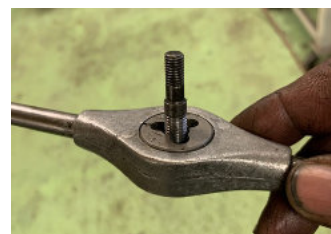
Using a die to clean up the threads. Even new manufacture parts, made to 0.0005" tolerance... may have burrs or small discrepancies. If they gall an aluminum casting, these discrepancies will cause time-consuming (and therefore expensive) issues!
