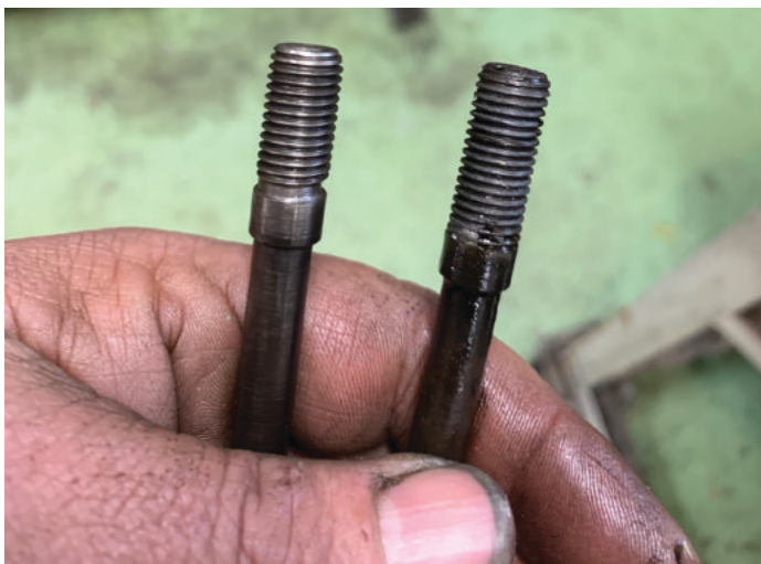
Another example of studs before and after chasing. Note stud on left is burnished, chamfered and has a clean groove under its shoulder. The right one is "out of the bin."
