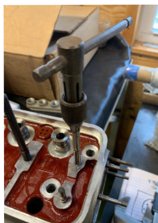
Using a tap to clean up the threads in the casting. Be very cautious here. Use new, sharp taps. Use kerosene or Tap Magic (Aluminum) for lubrication. Do not do this dry. Each hole should be carefully chased. Beware copper tubes behind the stud holes!
