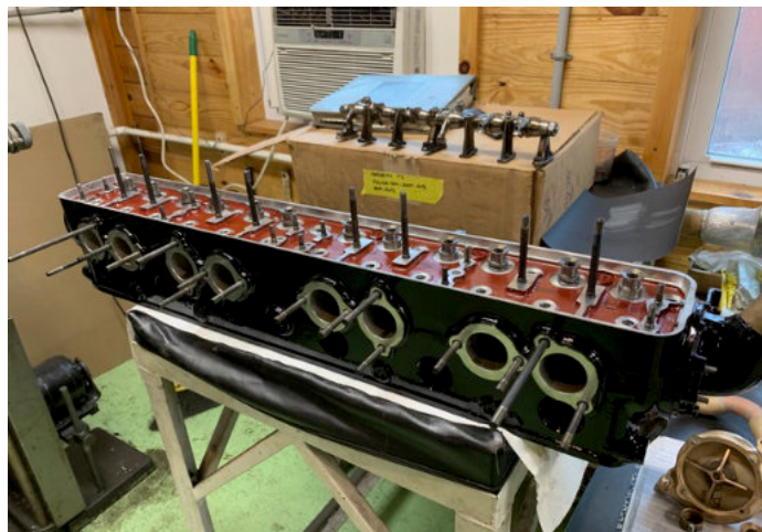
Head painted and ready for final fitting. We paint them in-house to match... ordering them from the UK unpainted. All studs in place, all parts test-fitted. You can now fit your head with confidence.
