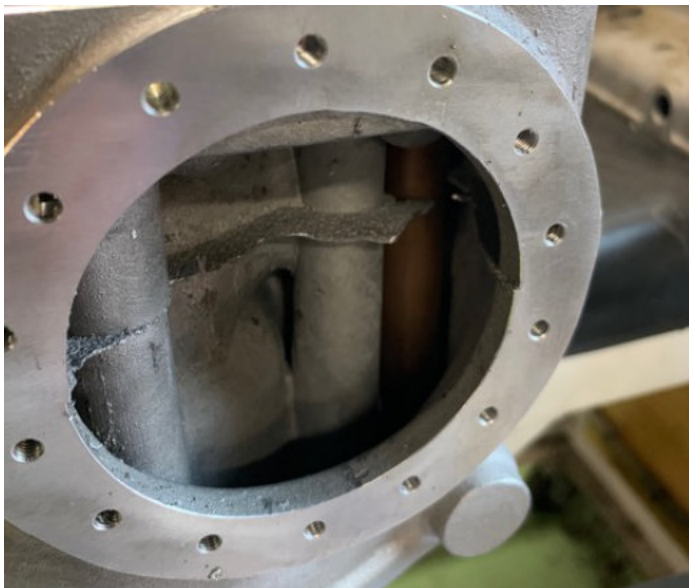
Upon inspecting the head, we found some pieces of casting flash... the 'shelves' sticking out from the casting. These are broken off and cleaned up where they can be reached.
