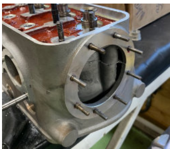
Front studs being fitted. Because the front cover has recesses for the stud shoulders (which align the cover), they protrude slightly. The excess Loctite will be cleaned off before fitting cover.
