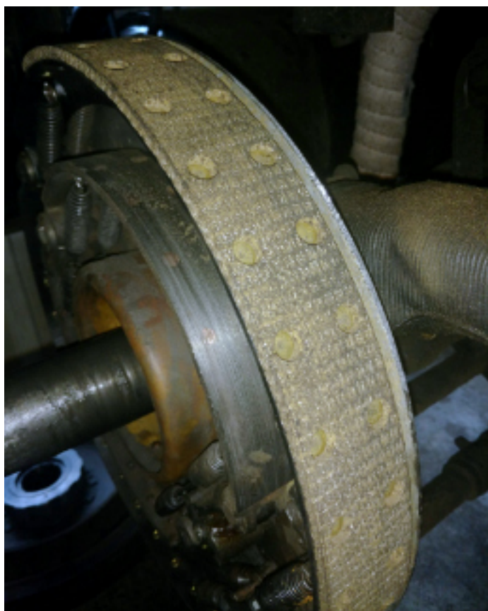
Check brake linings for condition and wear. Even with linings in good condition, braking can produce excess noise!
