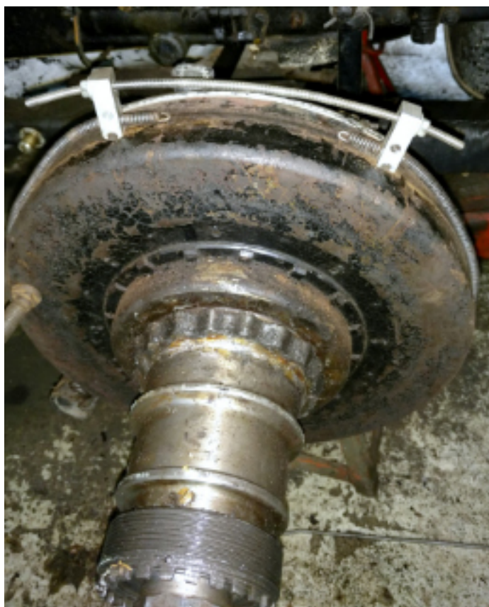
This device made up of a threaded rod and blocks that clamp the spring can make the installation and removal of the anti-noise springs much easier.
