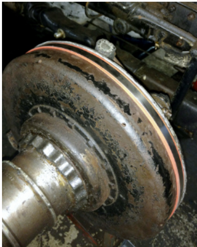
Installation of a thin rubber strap around the drum and secured with a stainless steel band that would clear the steering linkage resulted in elimination of noise.
