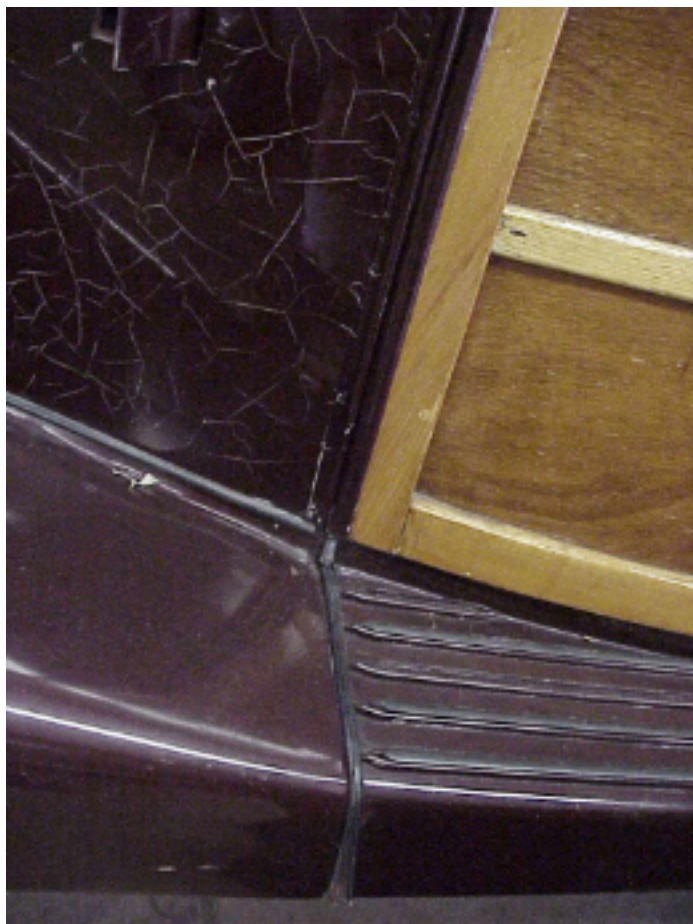
The paint was heavily crazed and the finish on the wood had deteriorated to the point that it required a full refinish.
