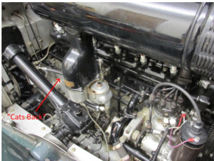
Engine compartment of GYD44 showing the “Cat’s Back” carburettor arrangement.
