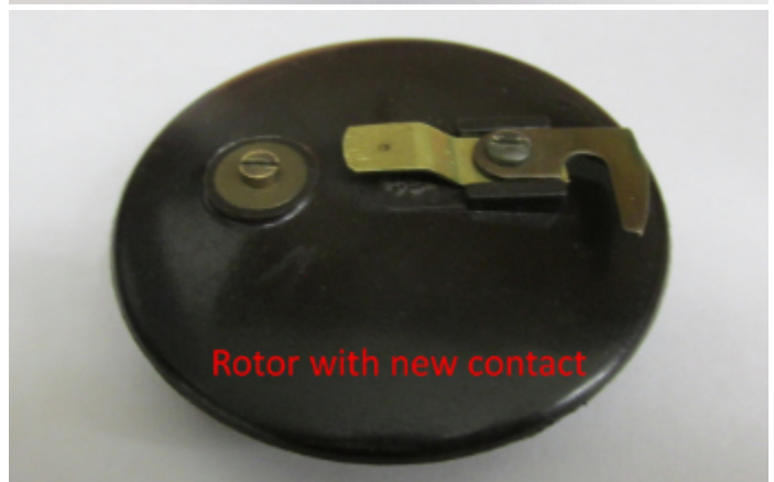
Top Photo: Blistered surface of the rotor beneath the contact. Bottom Photo: New contact installed with 1/8" gap above rotor surface.
