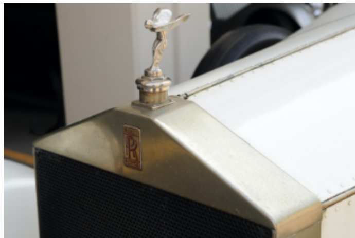
Mascot and radiator shell. Note that the shell has rounded edges, rather than sharp box edges. Photo: Gates
