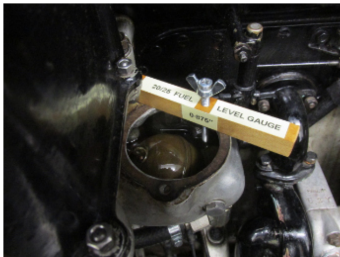
The author made this gauge to verify proper fuel level..
