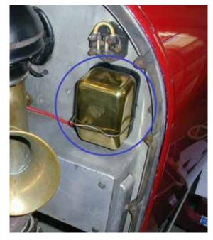
Next on the list was mounting the new regulator while affecting the car as little as possible. Our goal with any of these modifications on classic or vintage machinery is to make them easily reversible in case a return to originality is required. Thus we searched for bulkhead bolts or fasteners which could be pressed into service - what we found was the opportunity to make use of three existing drilled and
