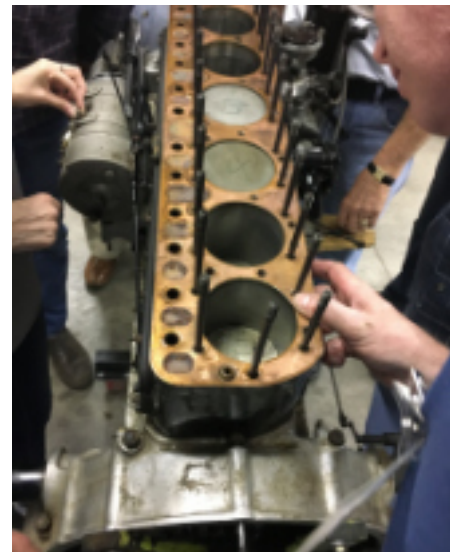
Cylinder block with head removed, looking at pistons with lots of long thin studs.
