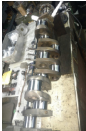
Above and Right: Measuring crankshaft main journals.
