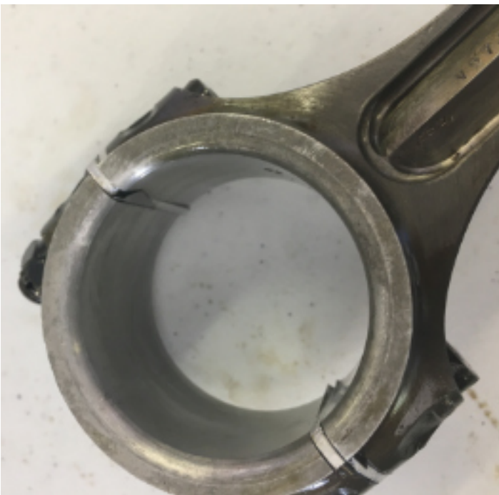
These incorrect thin steel shims had slipped and protruded past the bearing clearance and interfered with the crankshaft.
