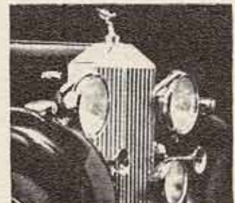
If the headlights are alongside the radiator, the car is a Phantom III (PIII).
