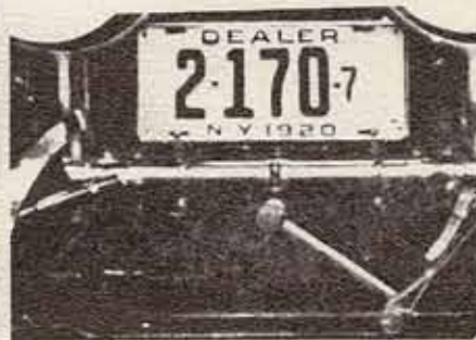
If it has a permanent crank, it is a British Silver Ghost.
