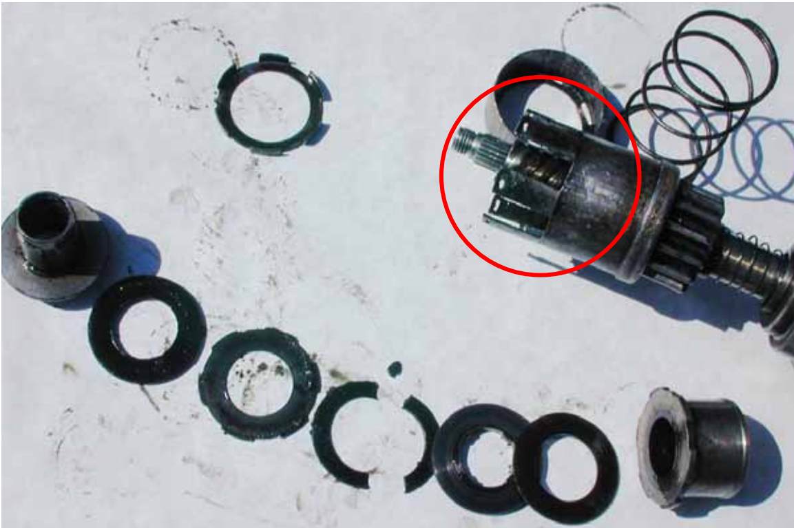
1. The rather sad state of the clutch discs on the 20/25 starter.
