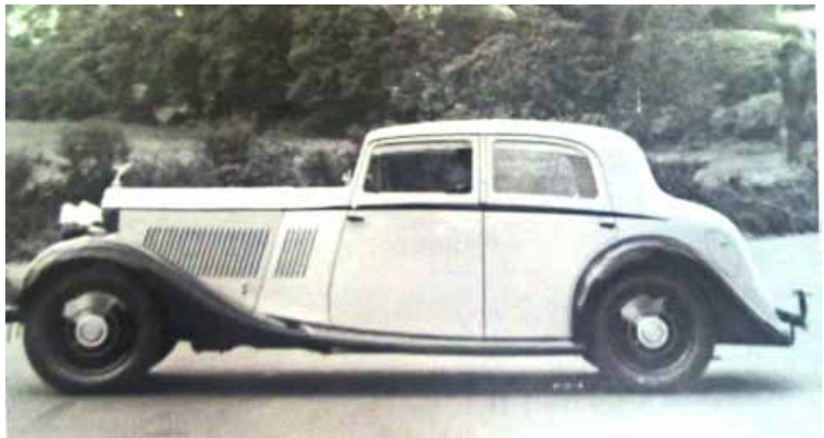
Original Hooper coachbuilders photograph of GPG23 showing the low roofline and continuation of the louvres through the scuttle, matching the windscreen angle, all combining to create an attractive low-slung profile.
