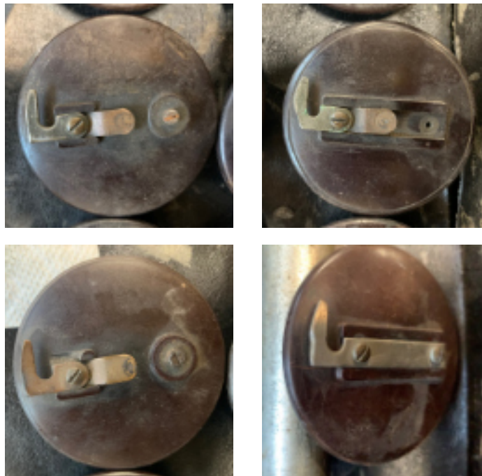
Distributor rotor contacts -- and the origin of the Nose vs. Tail debate. These show severe wear due to neglect of the distributor. Yet all came off 'running' engines. Though one could say that 'running' is a relative term. Photos: Reid
