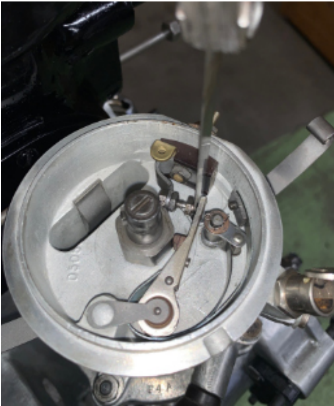
Small horsepower distributor gap being set with .018" feeler gauge. This is in your handbook. The points should be cleaned and reset regularly. Follow handbook recommendations for both mileage AND time. Your car came with a points file in the toolkit for a reason. Photo: Reid
