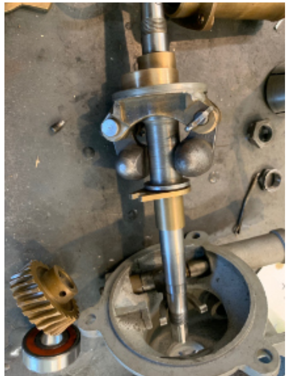
The Origins of the Small Horsepower Distributor are found in the Silver Ghost distributor, which uses a flyball governor. You can see the large cast-iron balls on pivots. As speed increases, balls fly outwards... balls to the wall. Photo: Reid
