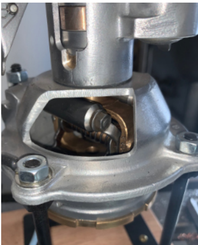
Here we see the flyball advance mechanism of the small horsepower distributor. It is much more delicate and complicated than the earlier Silver Ghost unit. But is a very effective mechanism using bar-weights on a scissor mechanism to control the advance. Photo: Reid
