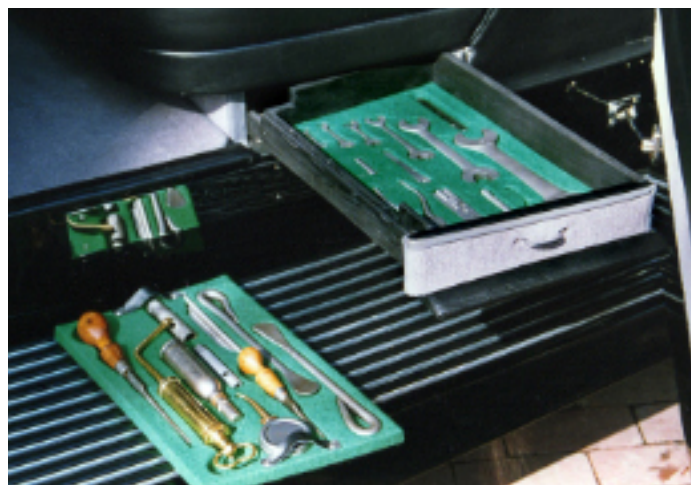
WHC43 carries a complete tool kit stowed in a drawer beneath the passenger seat. Photo Timmons.
