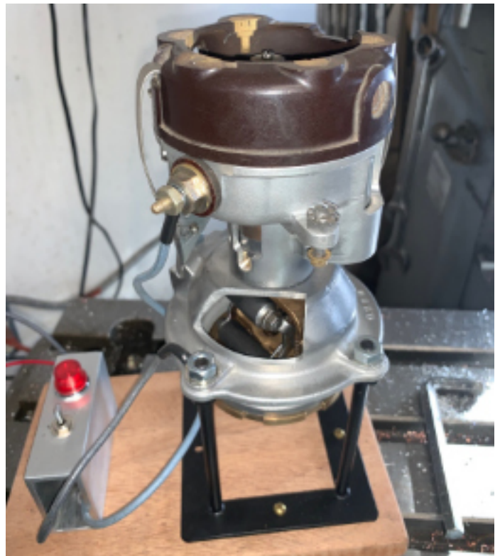
The Vintage Garage made this cutaway distributor as a demonstration to show the positions of all the parts at the exact moment when the points open, collapsing the field in the coil and making the spark. Everything must work precisely on time if the engine is going to run correctly. Photo: Reid
