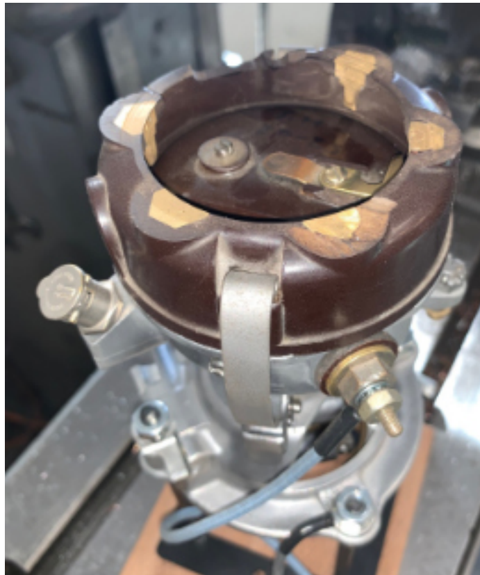
Cutaway governor showing the rotor in position. Each time the red light goes out on our demonstrator cutaway, the spark will 'fire' across the contact an up to the plugs. This lets us see exactly the point at which the points open and where the two contacts are in relationship to each other. For more detail, see the three YouTube videos linked to this article. Photo: Reid
