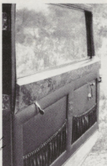
Two door handles are provided — one for the front seat passenger and a second for those in the rear due to the exceptional length of the doors.
